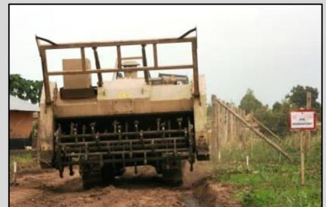
Mini MineWolf Demining Machine manoeuvring through houses
