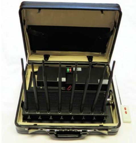
A sophisticated eight antenna (multi signal) jamming device built into a suitcase. One such "serious kit" was recently used by a British drug courier in 2016.
