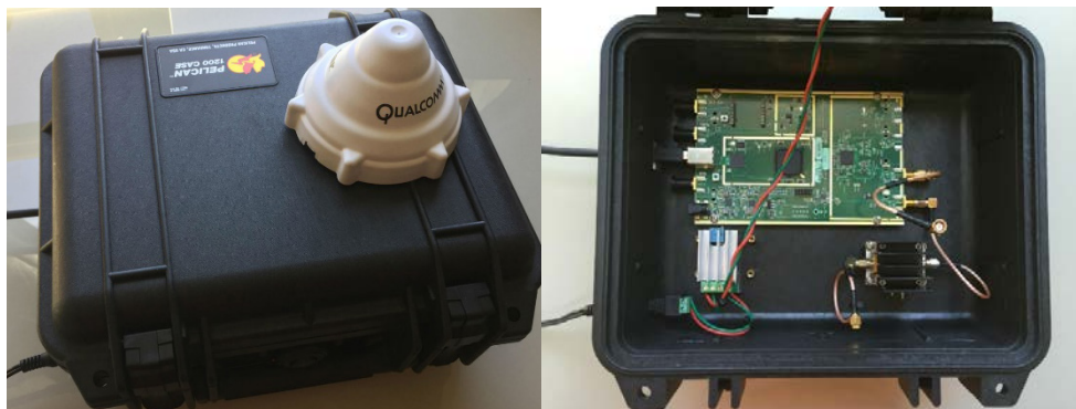
The device built by Synack to intercept data between GlobalStar tracking devices and its satellites (Colby Moore).
