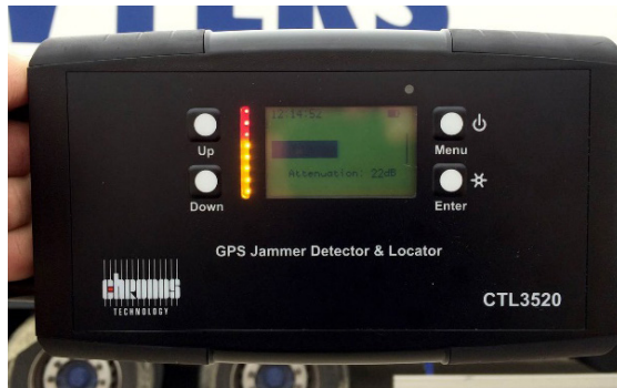
A device used by authorities to detect truckers using jammers (ChronosTechnology Ltd.)
