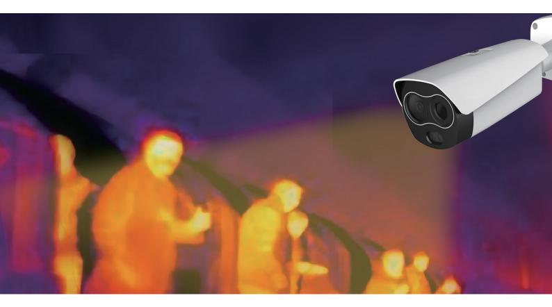
A vital tool in the detection of elevated body temperature which may indicate the presence of a fever, a symptom of the Coronavirus (COVID-19)
